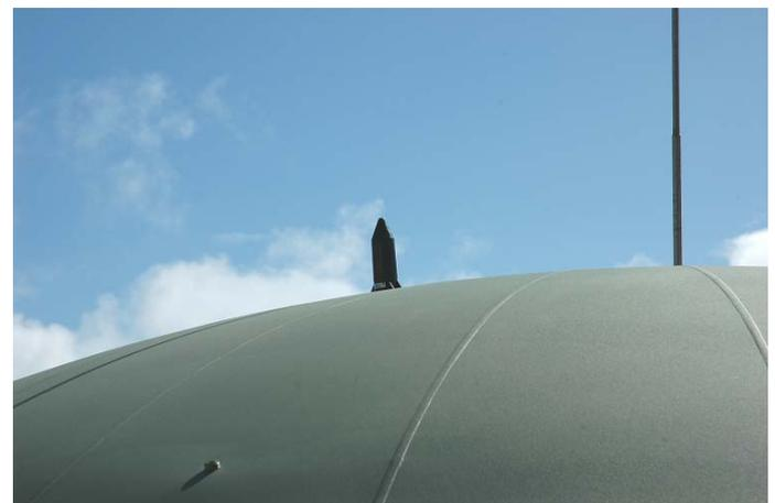
The Rain Alert™ wireless tank level monitor is fitted to a tank system at the RWRC and transmits a reading of tank levels to a Receiver located in the Engineering Faculty over 150m from the tank.
