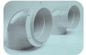
To fit Tank Outlets, simply rivet or screw onto the tank wall. If using screws, drill a hole in the fitting first. Rain Harvesting's Flap Valves and Mozzie Stoppa™ screens can fit directly into these outlets to insect proof the tank.
